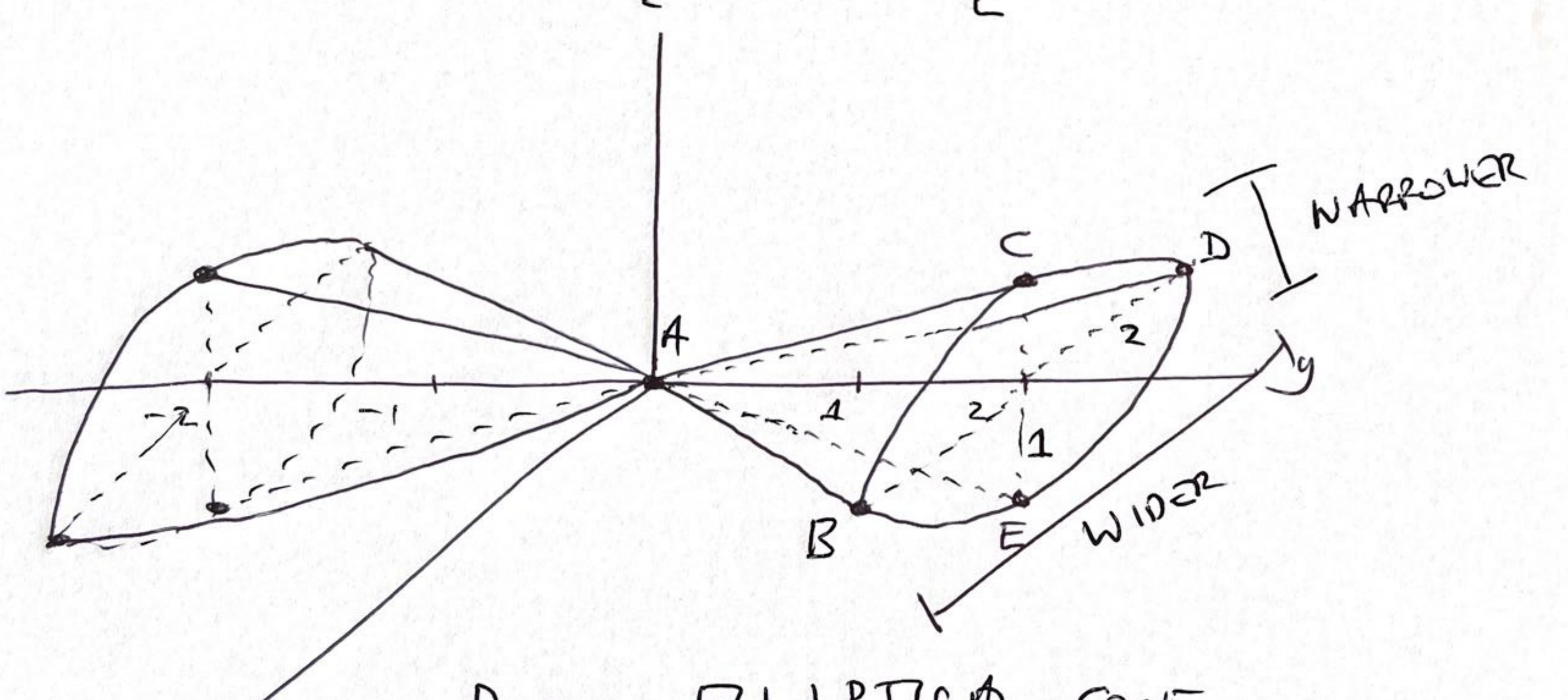
DOUBLE ELLIPTICA CONE ALIGNED WITH YAXIS.
